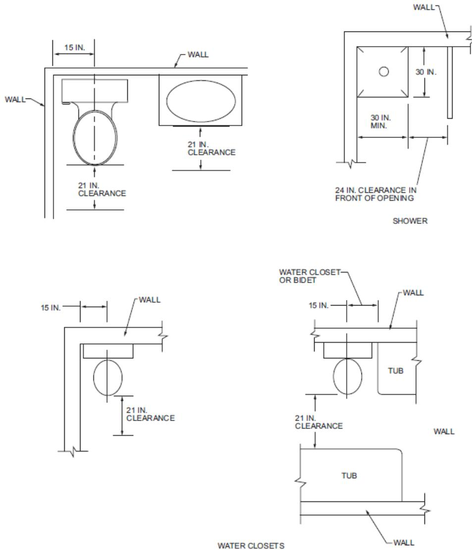
The 2018 International Residential Code governs for the location of the plumbing fixtures; however, the 2018 International Plumbing Code is used for the plumbing system installation.
